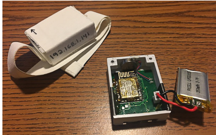
Fig. 5.5 Inside and outside of the prototype gesture control devices.
