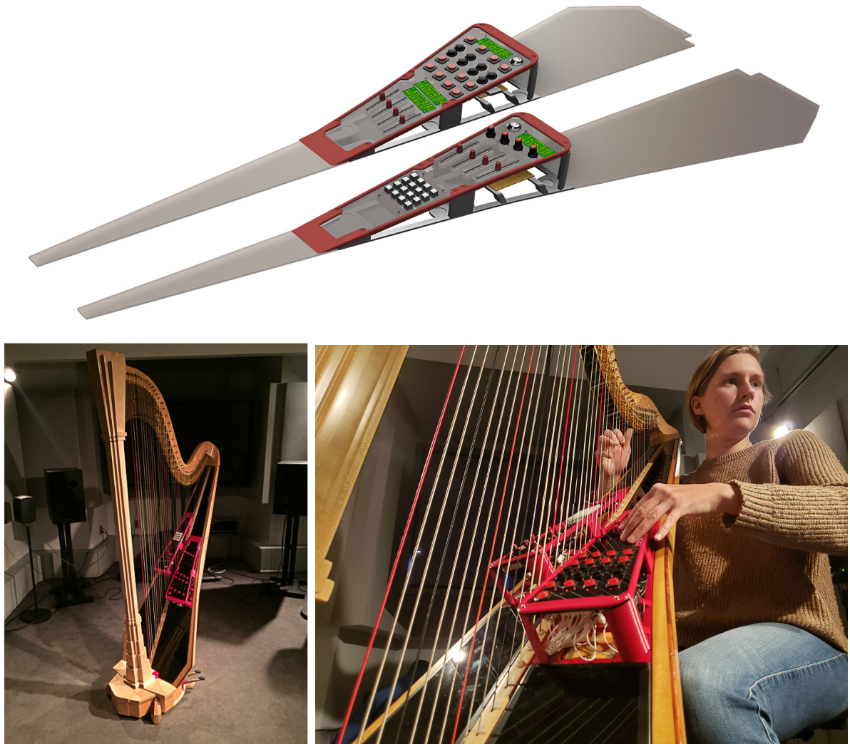
Fig. 5.11 Finished CAD model and fabricated controllers.
