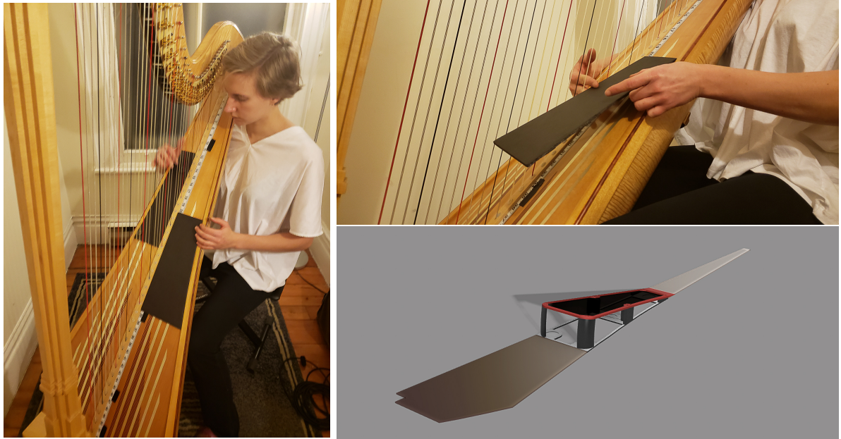
Fig. 5.10 Lo-fi cardboard prototypes allowed us to quickly identify unforeseen issues with positioning of interface panels and suggested alternatives that were converted into 3D designs.
