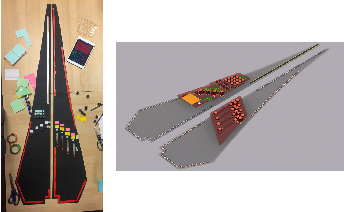
Fig. 5.9 Left: Non-functional prototype of interface panel layouts. Right: 3D model of the same panels.
