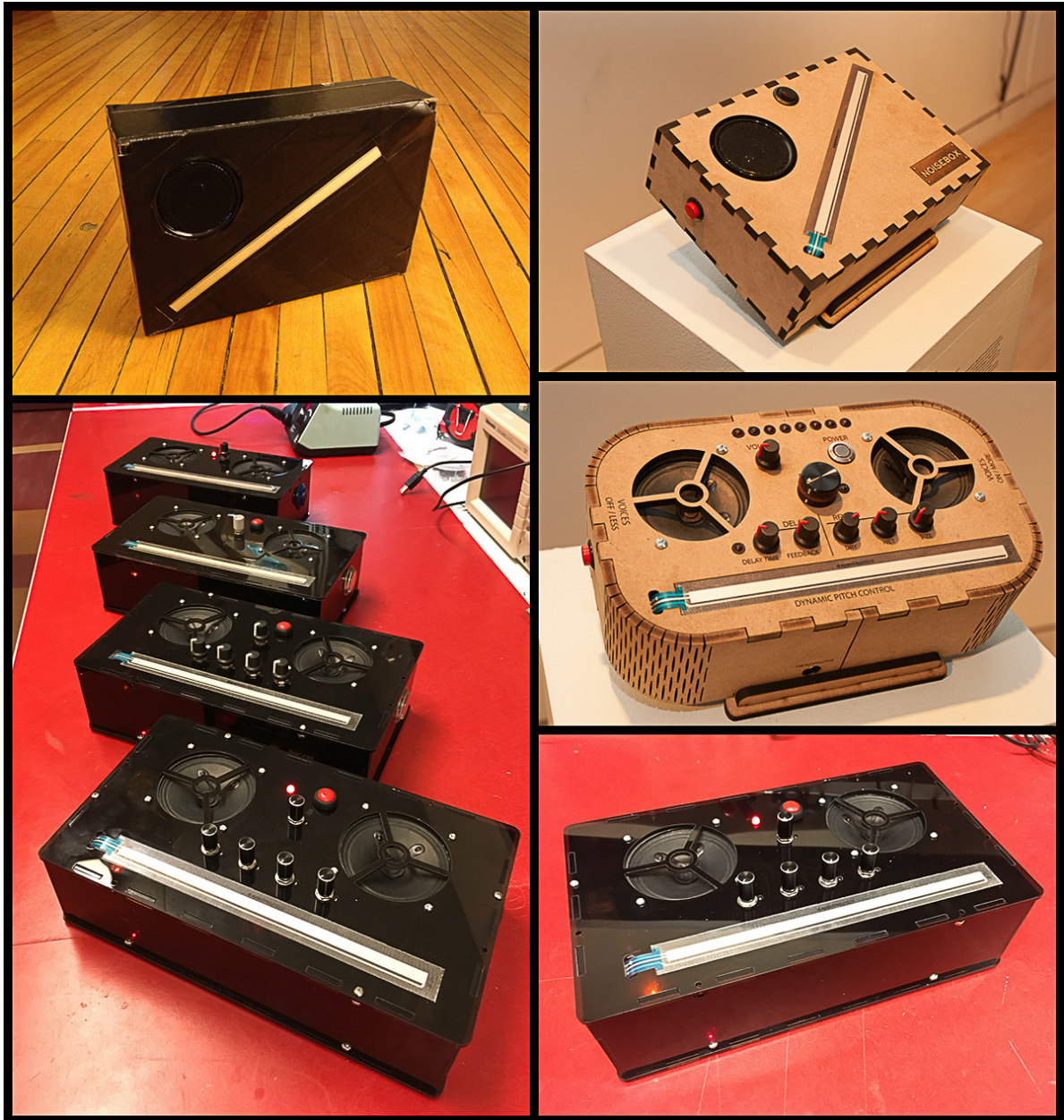
Fig. 4.1 The Noiseboxes, v1 & v2 ( Clockwise from top middle ): v1 initial prototype, v1 finished, v1 with additional controls and audio FX, v2 with additional controls and FX, a quartet of v2 instruments.
