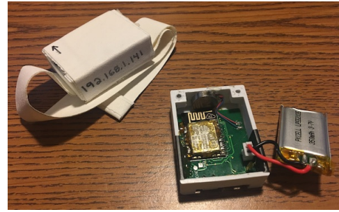
Figure 6: Inside and outside of the prototype gesture control devices.
