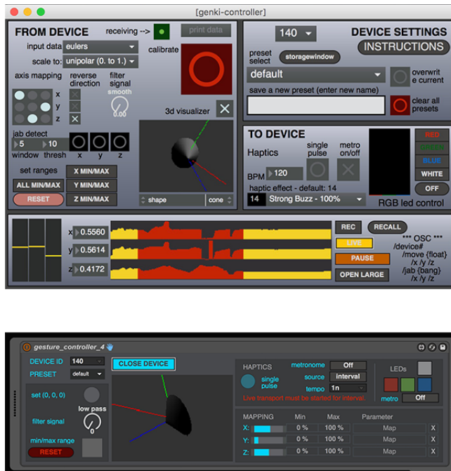
Figure 7: Top: User interface for Max and stand-alone use. Bottom: Max for Live device.
