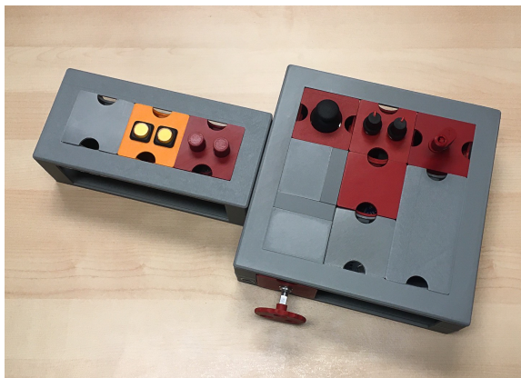
(a) A prototype constructed with a Probatio base, structural support and several control modules.
