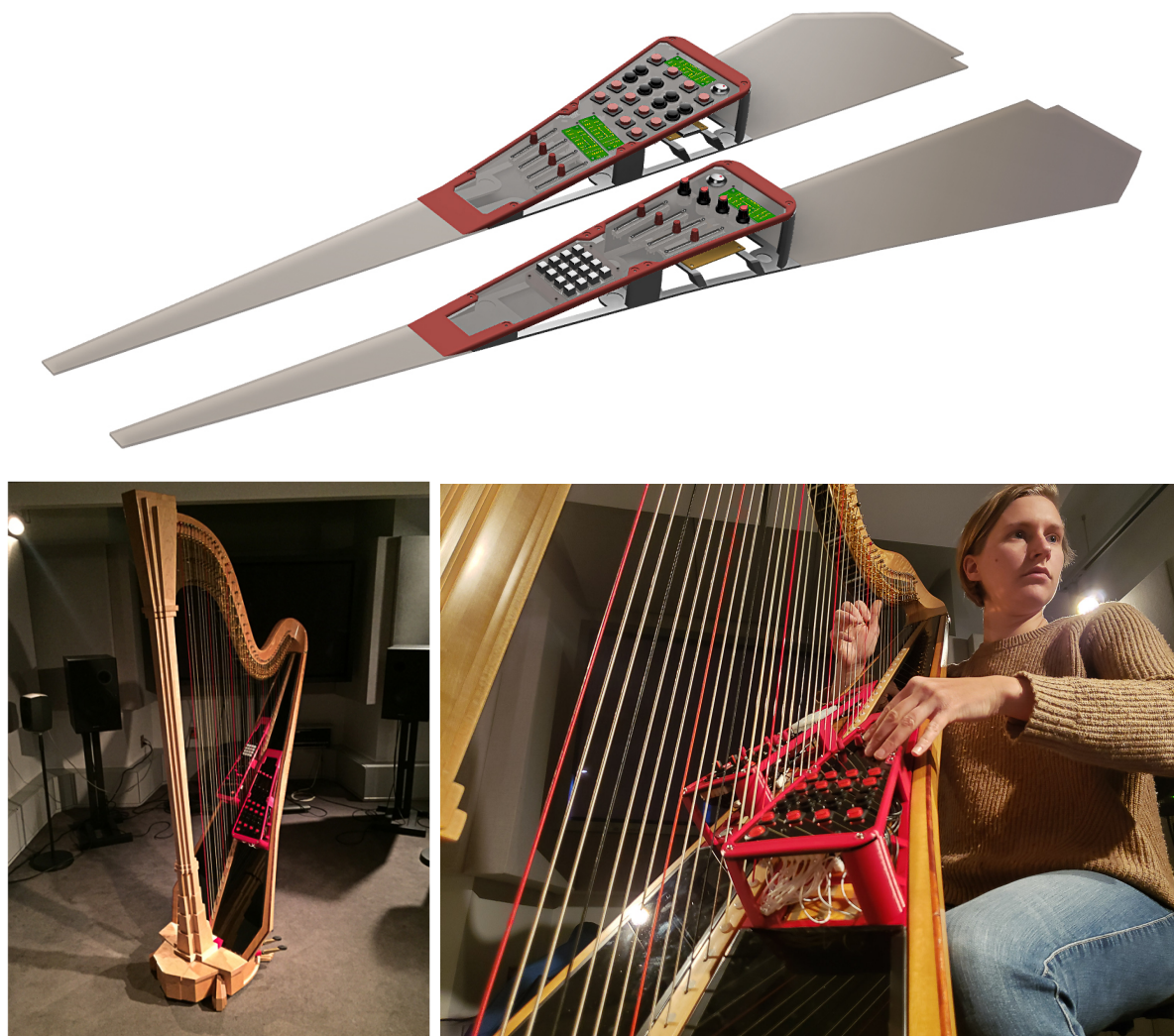
Fig. 5.11 Finished CAD model and fabricated controllers.
